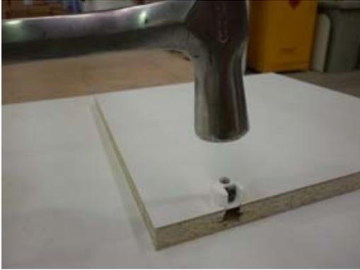
Hammer fix cam in place.
