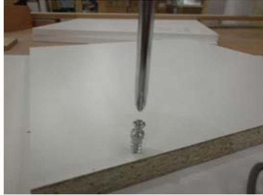
Screw fix cam bolt into 5mm holes.
