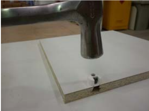
Hammer fix cam in place.
